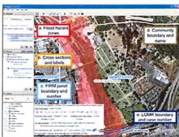
Figure 2. Results after “flying to” an address in Santa Cruz, California. The flood hazard information includes (a) flood hazard zones, (b) cross sections, (c) FIRM panels, (d) communities, and (e) LOMRs.
