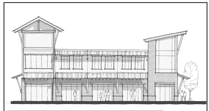
Articulated Wall Planes and Roof Lines
